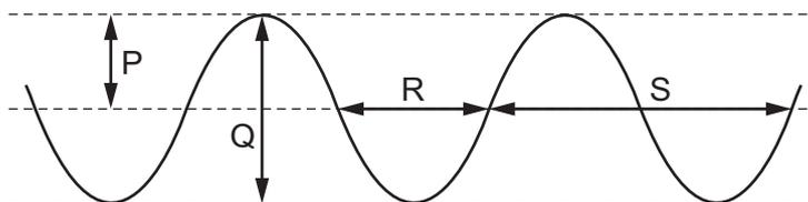
Which labelled arrows represent the amplitude and the wavelength of the wave?
